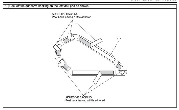
Attach the left tank pad as shown.
